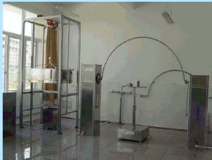
Drip tester, swing pipe tester
